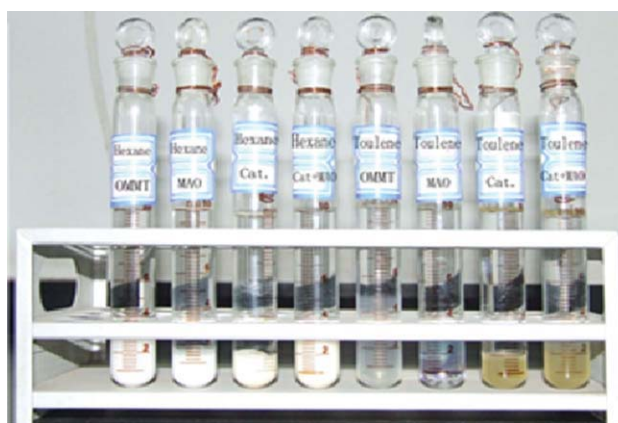
Figure 2 Dispersion and swelling profiles of OMMT, MAO, Cat. (Et[Ind] 2 ZrCl 2 /OMMT), Cat. + MAO in hexane and toluene, respectively.
